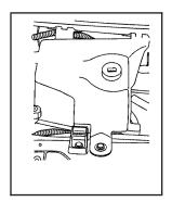
The coolant recovery tank is located near the center of the engine compartment. See Engine Compartment Overview on page 5-12 for more information on location.
